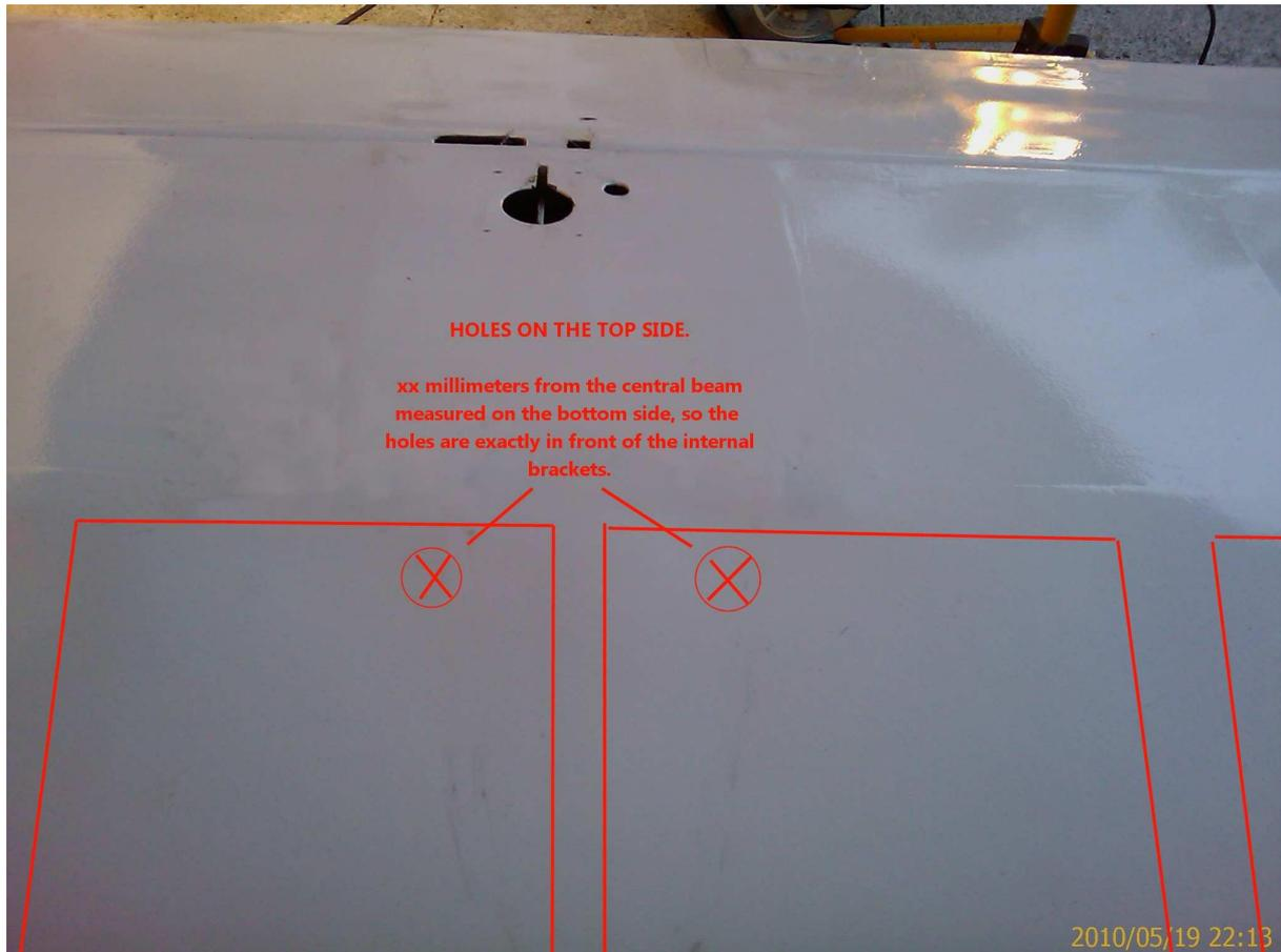
The above picture was agreed with the factory to be a good way to get inside for repair. The holes were first drilled 22 millimeters, but increased to 42 for access with tools.
