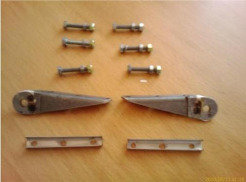
New M4 8.8 grade bolts, stainless steel all-metal lock nuts, and a stainless steel racks were fabricated and test mounted before gluing.
