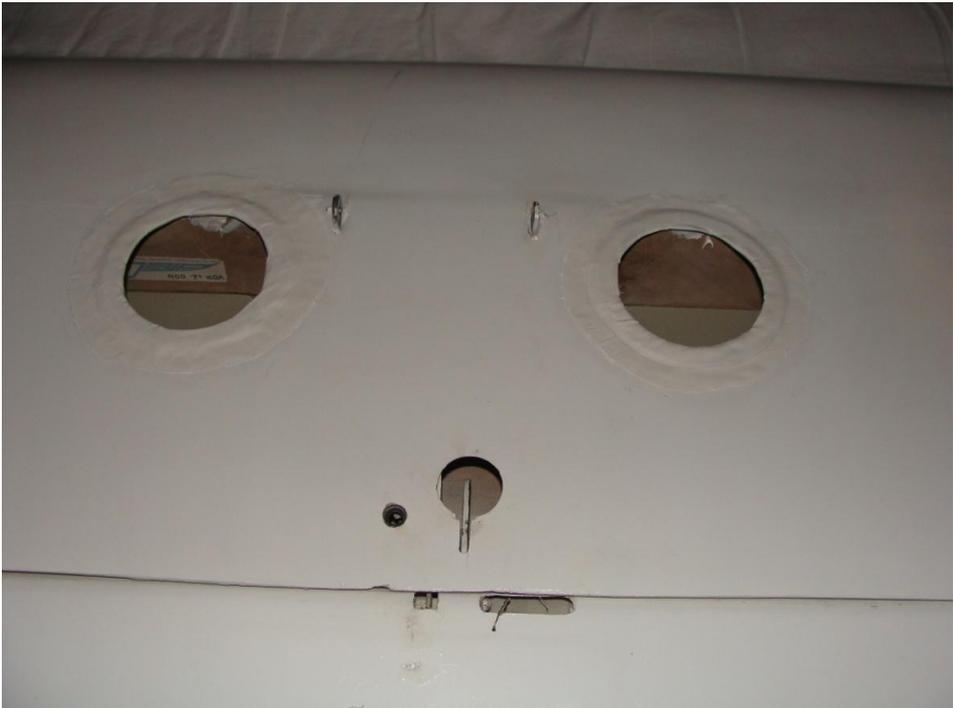
The rip stop rings were covered with a transparent lid of plastic, and covered with transparent 3M ControlTac 180 film. A visual inspection of the brackets can now be done without opening the tail wing again.
