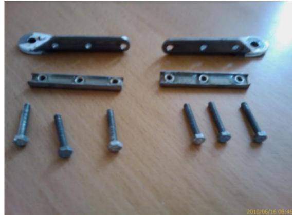
Racks and brackets were glued to the wooden beam when they were mounted with T-88. The nut did get a thin layer of copper paste to avoid bolts rusting or being glued to the nut. It also will make it possible to tighten the bolts if necessary at a later stage.
