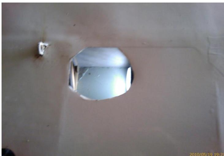
On the opposite side of the wooden central beam, hidden inside a D-formed torsion case, were the nuts used to connect brackets to the tail wing. The wing is made from a central plywood beam with a D-shaped fiberglass leading edge. This is a construction which does not allow the nuts to be accessed without cutting a hole.
