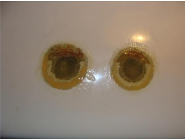
The Lamination was a little thicker than the original. This is not always better, but the 1mm lower glued fiberglass did make the first laminated layer a little thicker.
