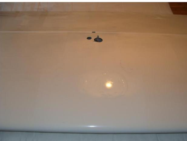
The inspection holes on the underneath were created using rip stop rings from AircraftSpruce. This makes it possible to inspect and do maintenance at a later stage.
