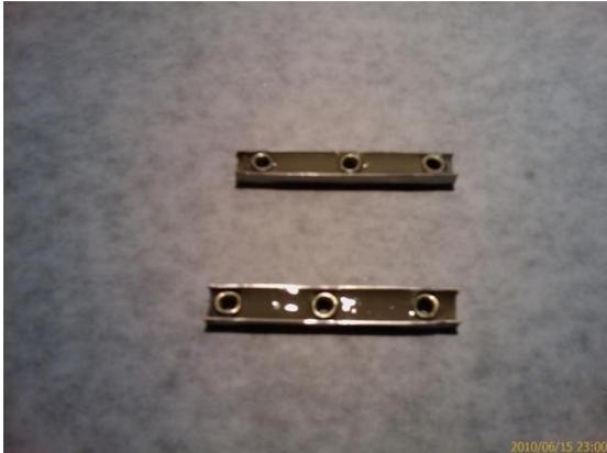
The racks were after gluing test fitted with brackets and bolts to ensure a good fit inside the tail wing.
