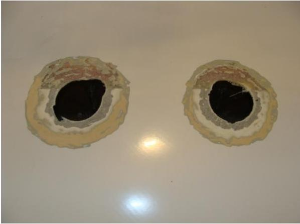
The picture shows the holes after the sanding. Every layer of the D box has been revealed. Since there is no possibility to glue from beneath, a layer of glue was smeared on the underside of the holes, and the first ply of fiberglass were pushed 1 millimeter into the hole so the lamination was in contact with it.
