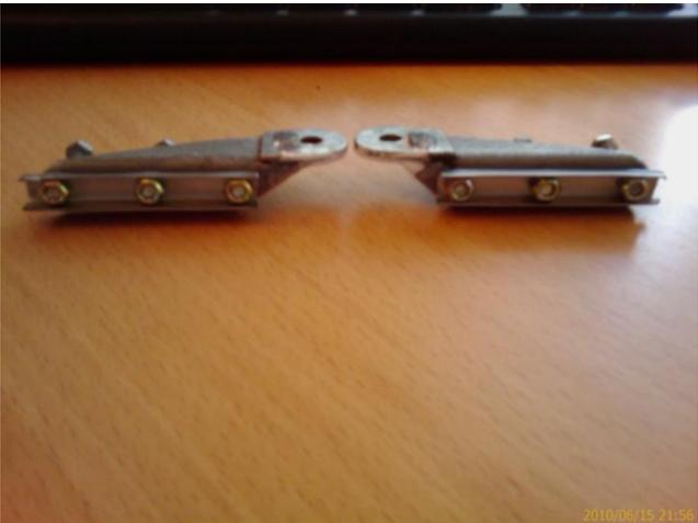
The racks are made from 1.4 millimeter stainless steel, as a tray which can hold the 7mm nuts rather tight. The nuts were glued into the rack with cyanacrolate glue, before T-88 epoxy was used to fill all space between the nuts.
